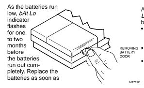
possible after the indicator starts flashing. If you do not replace the batteries when the indicator light is flashing *bAt Lo*, the indicator stops flashing. When the batteries are almost completely dead, bAt *Lo* stays on without flashing to indicate the thermostat and heating/ cooling system have stopped working.
